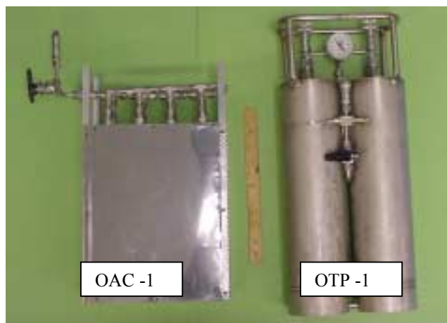
Figure 1: Ovonic prototype OAC-1 and OTP-1 metal hydride hydrogen storage modules.
