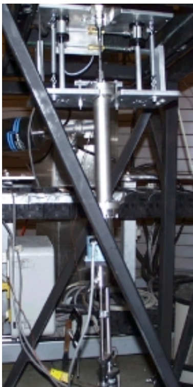
Figure 13. Particle Feeding System (below reactor assembly)
