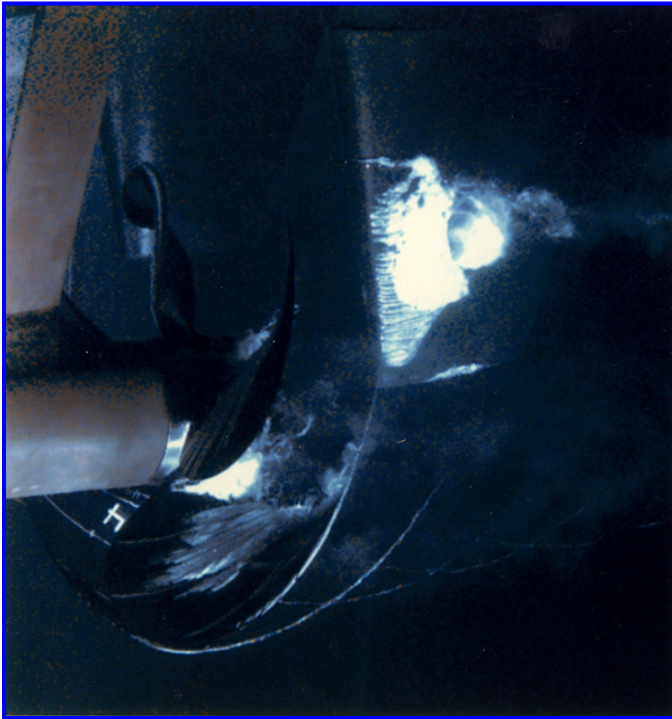
Severe rudder cavitation in a LCC test
