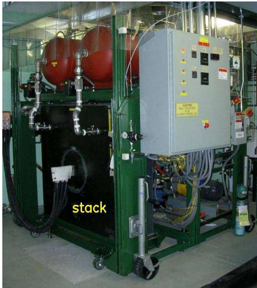
Figure 8: 1 kg/hr ambient pressure stack in GE test facility
