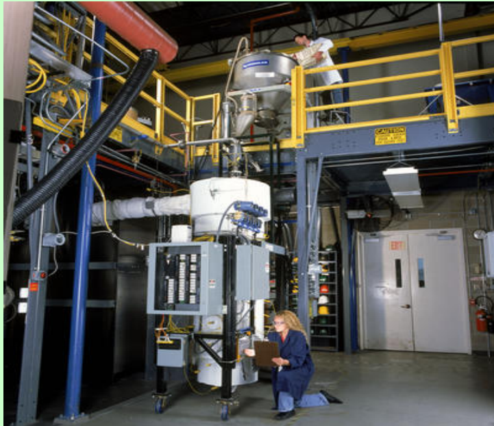
Biomass gasifier/pyrolyzer PDU (NREL)
