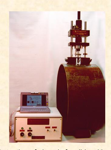
System that will be reassembled at ORNL for mechanical testing at hydrogen pressures upto 5000 psi
