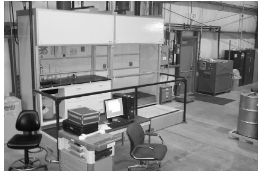
Fume Hood for installation of SO 2 anode-depolarized electrolyzer tests
