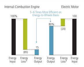
\* Energy loss includes loss due to heat, idling, driveline and electric resistance. Source: Toyota, U.S. Environmental Protection Agency and AllianceBernstein
