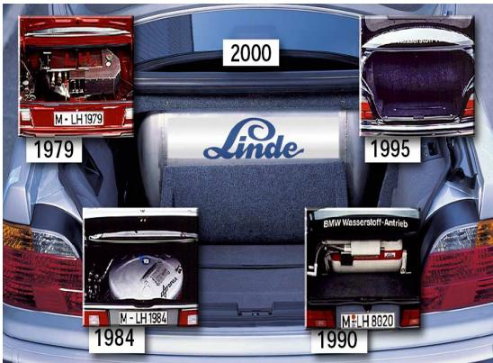
**Liquid:** develop conformable containers that can operate at extremely low temperature (20 K) and wide range of pressures (100-5000 psi)
