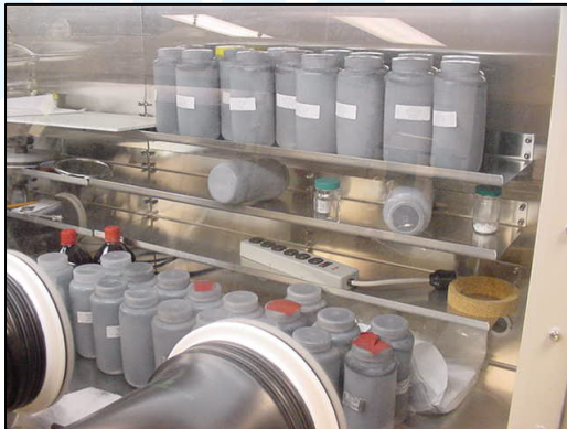
Media handled & stored under inert gas
