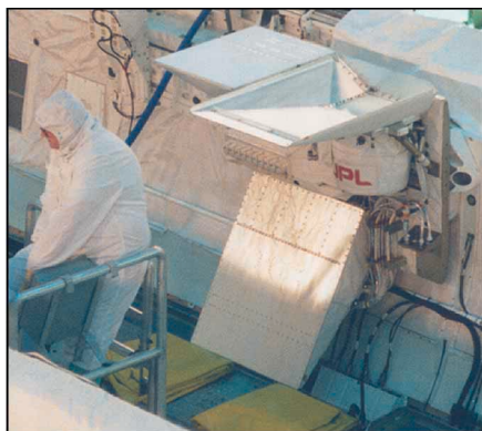
Figure 7. BETSCE (brilliant-eyes ten-kelvin sorption cooler experiment) hydrogen-sorption cryocooler mounted on the bay wall of the space shuttle Endeavor prior to flight in May 1996. Metal hydride sorbent beds containing \text{LaNi}_{4.8}\text{Sn}_{0.2}\text{H}_x and \text{ZrNiH}_x (hidden by radiators behind the technician) were used to produce first liquid hydrogen ( T = 27 K), then solid hydrogen ( T = 11 K) in the cryostat (covered by the blanket with the JPL logo).
