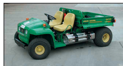
Figure 6. A John Deere Gator utility vehicle modified by Westinghouse Savannah River Co. and Energy Partners to operate with proton-exchange membrane (PEM) fuel cells and hydrogen gas stored in hydride beds (the cylinders mounted in front of the rear wheel). (After Reference 25.)
