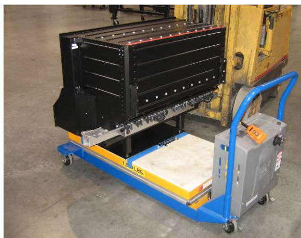
Figure 1 – Tesla Roadster battery pack
