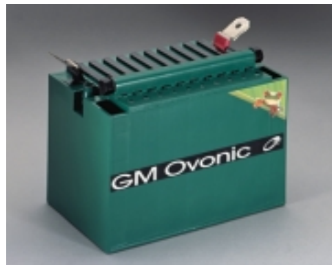
Figure 4. Water Cooled Ovonic NiMH Module (10 cells, 12 V, 12 Ah, 48 Whr/kg, 550 W/kg)
