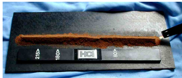
Figure 1. Photograph of the safety test set up measuring powder burn rate.
