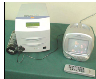
Figure 10: 50 W MHFC demonstration system
