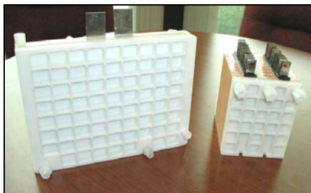
Figure 8: 250 cm 2 single cell (left) and 60 cm 2 stack (right)
