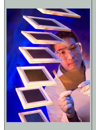
Kevin Fok, manager of marketing, holds the innovative hydrogen electrode from the Ovonic Metal Hydride Fuel Cell, a fundamentally new type of fuel cell that can store electrical energy inside the fuel cell stack. This new technology from Ovonic Fuel Cell Company has the potential to revolutionize power systems due to its unique performance advantages, including onboard energy storage, instant start, and good low-temperature performance.
