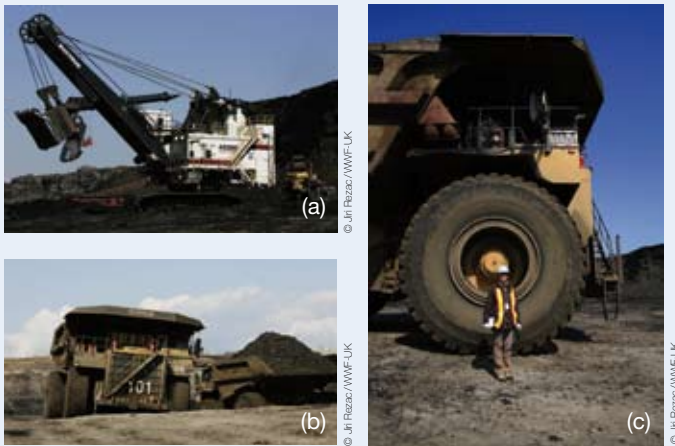
Figure 13. Oil sands in action: (a) hydraulic shovel moving 40 m 3 of earth with every scoop; (b) 'monster trucks' on the move; (c) the wheel alone is 4 m tall.
