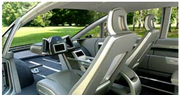
The Hy-Wire features handle bar controls that can be moved to either front seat.
